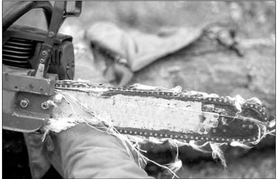
The above photograph illustrates how the basket-woven Kevlar fibers stretch across the chain's cutters. This, in effect, slows its penetration, allowing increased reaction time.
