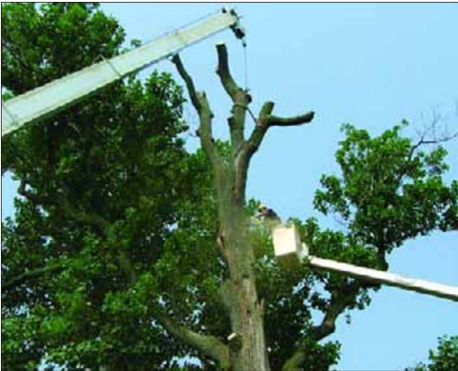
Never use your aerial device as a crane or a hoist unless it is designed by the manufacturer to do so. Continued operations that exceed the load limit of the basket will lead to failure of the upper boom.
