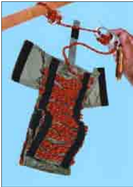
During the Vietnam War, Hobbs developed a rappelling kit for pilots who might find themselves stuck in the forest canopy. The prototype contained a miniature Figure eight, a carabiner and rappelling line packed into a self-deploying bag that strapped to the thigh of a pilot's flight suit.
