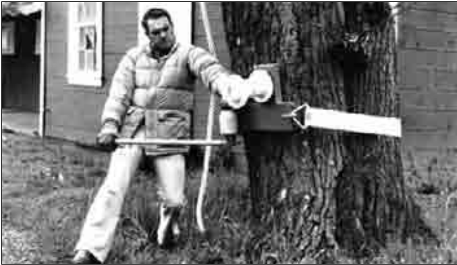
The earliest prototypes of the Hobbs Lowering Device began with a fixed spool.
