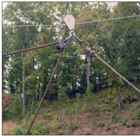
The wire rope running across the top is the speed line. The speed line pulley is on the wire rope. The carabiner on the left side of the eye of the speed line pulley is attached to the Pro-Traxion. The rope running through the Pro-Traxion is the pull rope. The left side of this rope is tied to the skid steer and the right side (hanging down) is tied to the material (wood/branches). The two carabiners on the right are attached to the control/haul back line.
