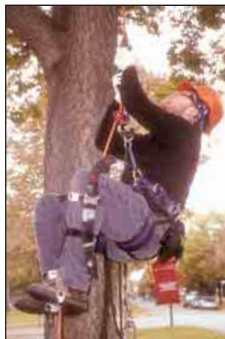
Placing the handsaw on a leg scabbard makes it much easier to access while in the tree.
